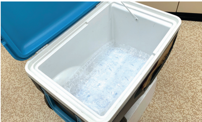
Figure 3: Insulating material placed in bottom of cooler
